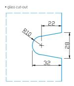
Suitable for glass wall from 8 to 10 mm
