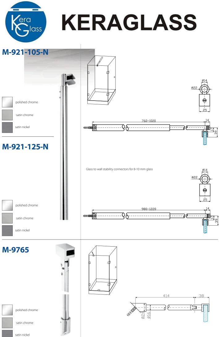
Glass to wall stability connector for 8-10 mm glass
